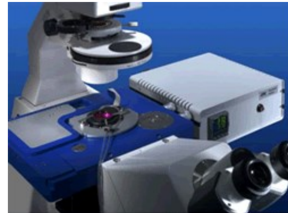
BioAFM incl. Petri dish heater for in-vitro imaging of cell cultures
