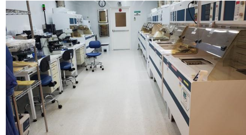
Wet Process Stations
