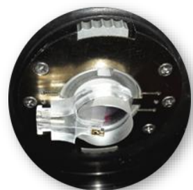
Cantilever holder with Cyto clip mounted on AFM head
