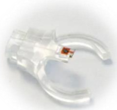
Cantilever holder with Cyto clip mounted on AFM head
