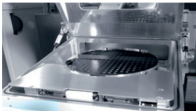
Fully automated 8 inch loadlock
