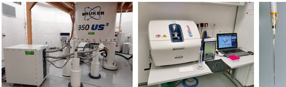
Figure: 950 MHz NMR spectrometer (left), EPR spectrometer (middle), NMR tube with cells connected to bioreactor (right).
