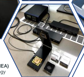
NanoIndenter Indentation of soft samples
