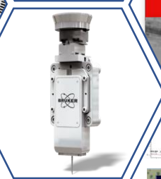
NanoIndenter Indentation of soft samples
