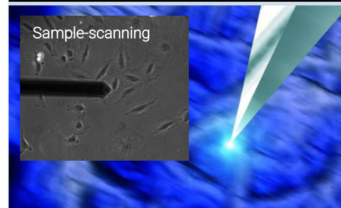
While scanning the surface, a sample scanning AFM moves the sample holder.
