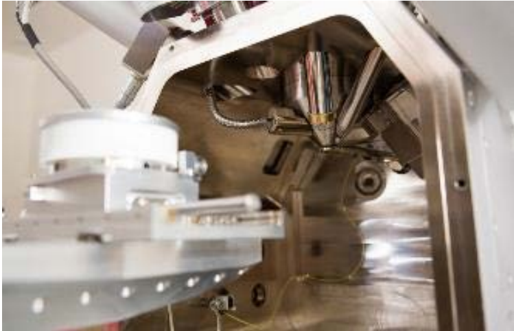
Scanning electron microscope with EDX and WD spectroscopy
